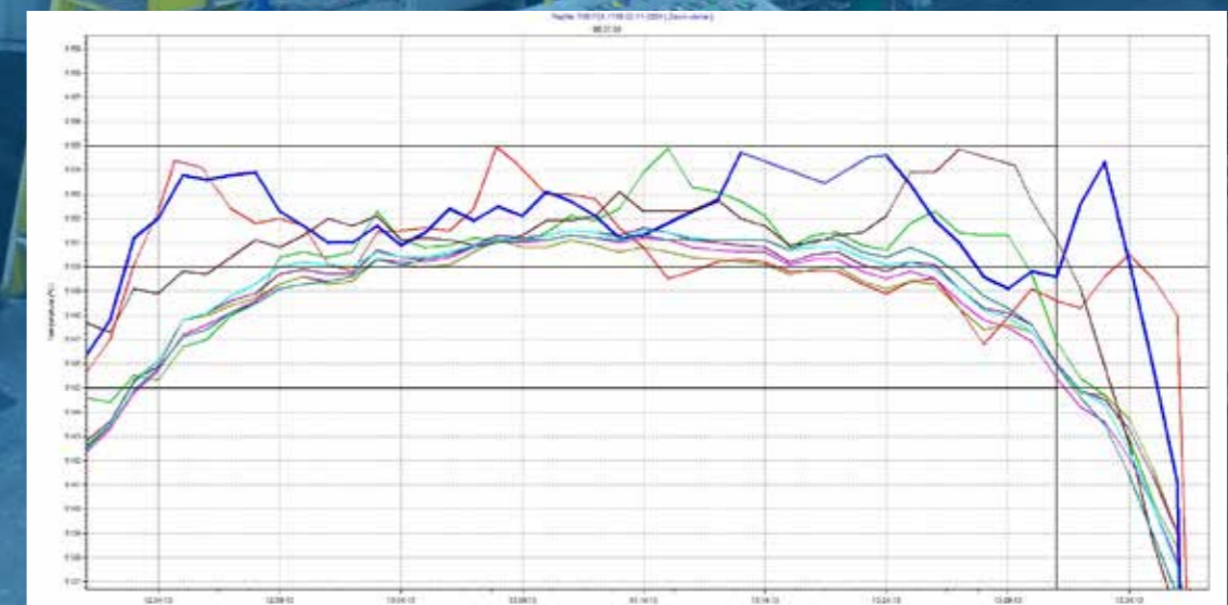
TUS at 1,150 °C (AMS 2750H class 2, dwell time of 30 minutes in the soaking zones)
