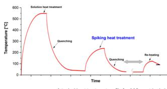
A typical heat treatment profile for AA6xxx strip during processing in a CASH line with additional spiking heat treatment
