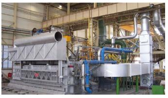
The completed shell of the 145 t dual-chamber melting furnace
