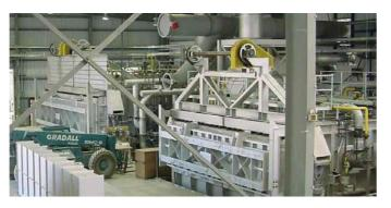
A pivoting 50 t scrap melting and holding furnace
