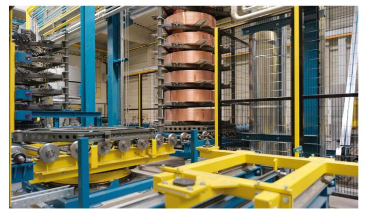
Fully automated coil handling and stacking station (Ingenia)
