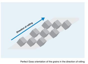
properties in the direction of rolling, due to a preferential orientation of the grains. The strict orientation of the easily-magnetizable grains, known as "Goss" orientation (see figure Perfect Goss orientation of the grains in the direction of rolling), makes the magnetization processes in the direction of rolling very favorable in terms of energy.
