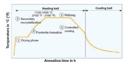
Schematic representation of a HITT annealing cycle and its component phases
