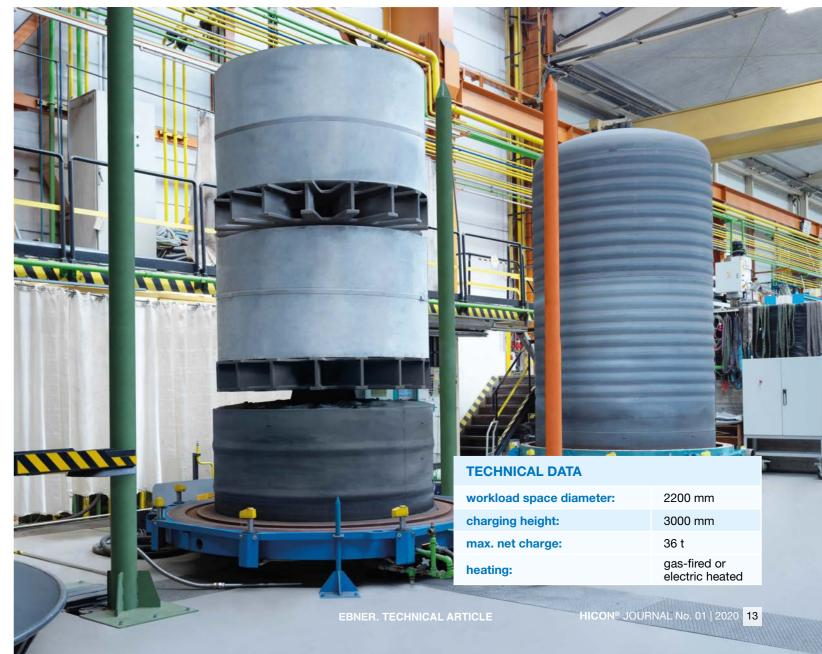
HITT high-temperature bell annealer (HBAF) charged with 2 GO coils
