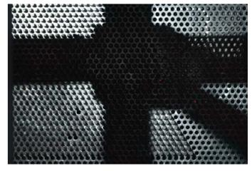
Top view of the cooling section of a press hardening furnace
