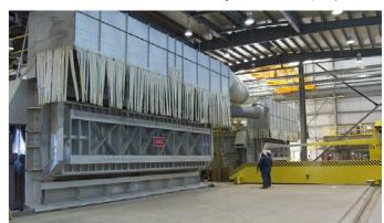
Melting furnace with a capacity of 18 t/h
