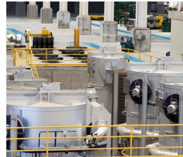
HICON/H<sub>2</sub>罩式退火炉
